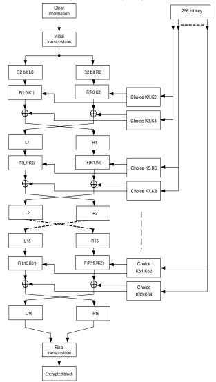
Fig. 1. Overall block diagram of the encryption algorithm
